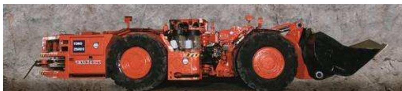
Figure 2: Side view of the Tamrock Toro 2500 electrical wheel loader; length: 14 meters, operating weight: 76 tonnes, and capacity: 25 tonnes.
